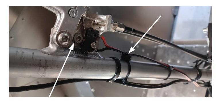
The little stop screw is not always needed. It can aslo make the brake sensor harder to move. You can remove it if necessary.
