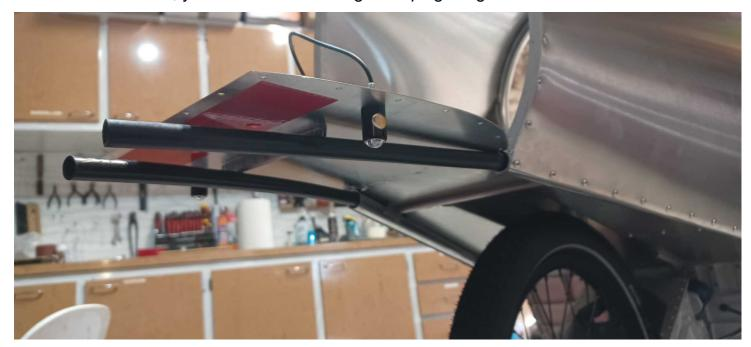
The rear light have to be fixed with the twin adhesive tape. You can also use the supplied screws if necessary.
