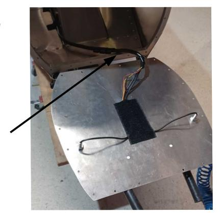
When the position of the cables is optimal, fix them with velcro. You can heat the velcro a little to make it stronger.
