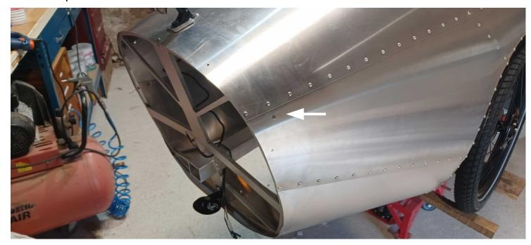
Fix the blinkers with the light side forward. Fix them with the m6 nut and threadlock. Be carefull about the little connections, when insert it trough the m6 nut (one after one)
