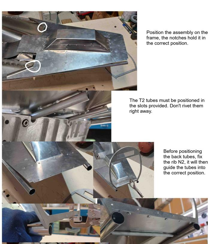
You can now complete the riveting along the tubes. Depending on the version of your kit, the holes must be
