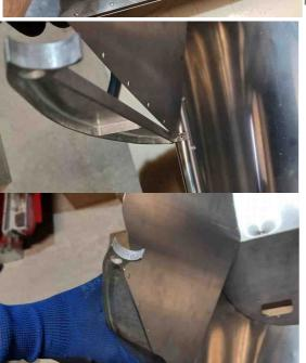
Fix rib N8 on the tube then bend it slightly to align it with sheet A8. fix the remaining rivets.
