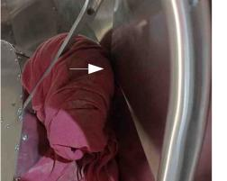
From the inside, place a rolled up cloth to maintain pressure against the sheet metal and achieve a regular convex shape.
