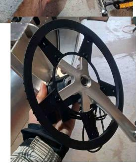
Mount the pedals, classic thread on right side, reverse thread on left size. Place the bracket holder on the boom and secure it with the aluminium clamps and R6x35 screws
