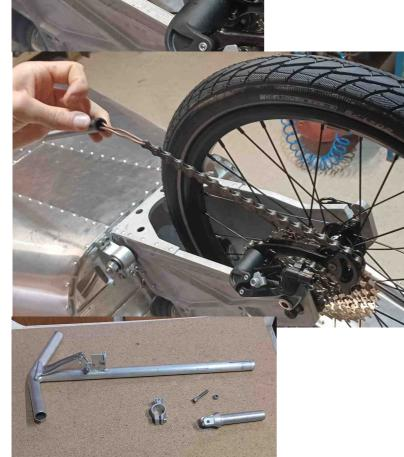
Tighten the collar firmly. The handlebar will not be completely locked, after road tests you can add a rivet to fix the position.
