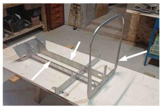
Bolt the main rib N9 with the sides N5. The parts should be positioned with the machined faces towards the rear or towards the sides.
