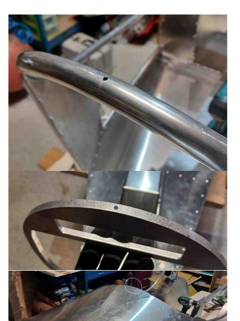
Drill a hole (rivet size) at the top of the back of the T2 tube
