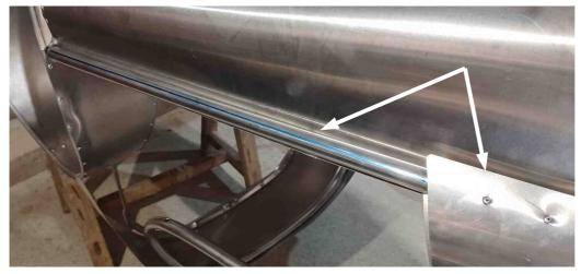
Trace the tube following the axis of the rivets already in place
