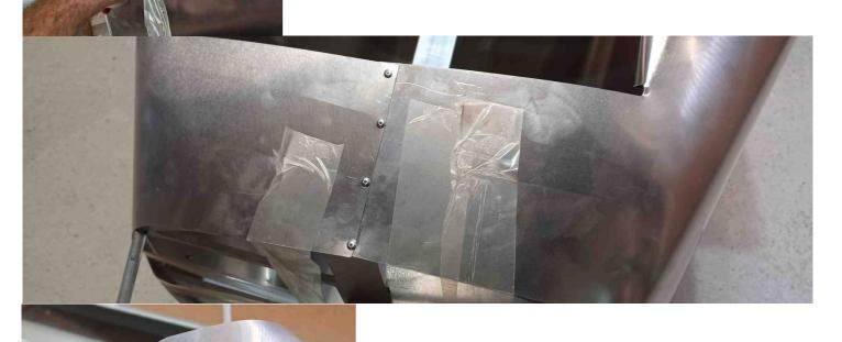
Fold the edge of the sheets against the wheel arches and add 2 rivets You can now draw the marks and finish drilling the wheel arches.
