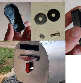
Make a hole in the bottom of the cover and insert the screw P5x16
