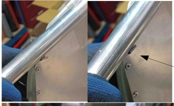
The ends of the supports should be bent slightly to fit the tube
