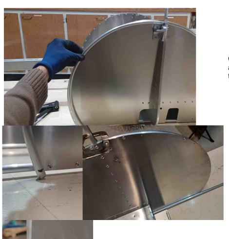
Continue with the T6 tubes. adjust, cut the excess and fix them.
