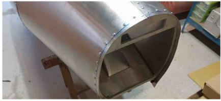
Don't forget the back part. Cut the sheet flush with rib N2
