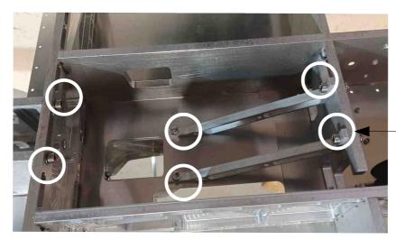
These 2 screws are on the back side, fiw them with 2 nuts M5f + W5
