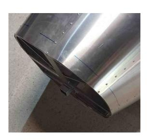
The trace tells you the distance the nose is covered. The cut must leave a minimum of 15 mm to allow the installation of the rivets.
