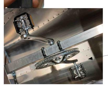
Place the pedal board in the middle of the boom without tightening the clamps.
