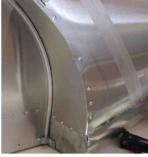
Attach a few rivets to the bottom of the wheel arch
