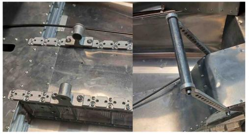
Rivet the S5 bars then install The S3 supports (P 6x12 screw + W6 washer)
