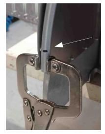
Set a starting point by marking the location of the first hole, then hold the tube with vise pliers.
