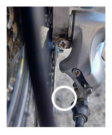
If the screw is too much tighten, the derailer idler will be far from the cassette and will loose some precision when shifting
