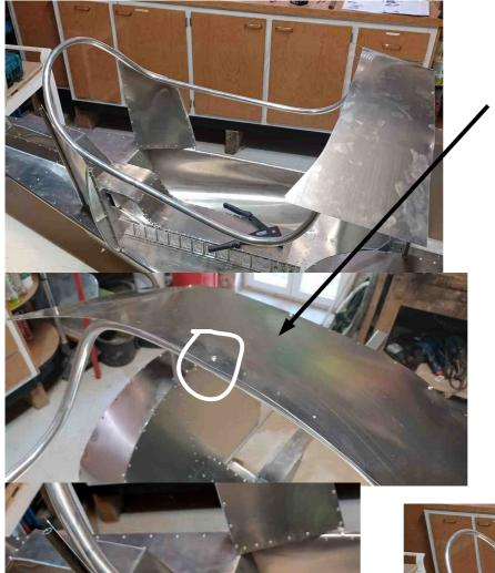
Present the tube on the frame. Fix the central rivet on the front part
