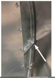
The N8 ribs have a reinforcement in the middle. The rivets must not fall out!
