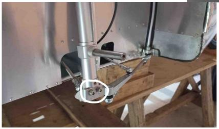
Secure the steering bracket to the suspension with two screws R6x16 + W6 washer, add threadlocker
