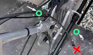
Pass the outtercables through the cable grommets in the floor.
