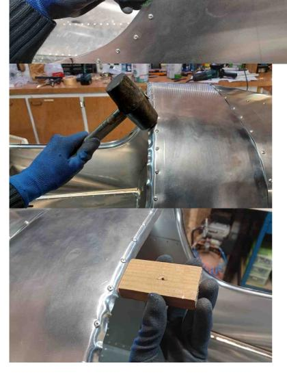
Start to hammer the sheet metal gradually by multiplying the passes. Continue using a wooden block to remove the wrinkles.
