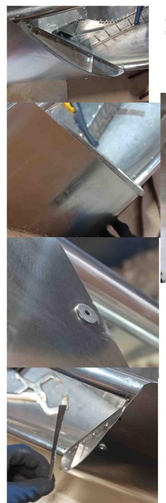
The N8 ribs may not be perfectly aligned with the sheet metal, adjust them by hand if necessary.
