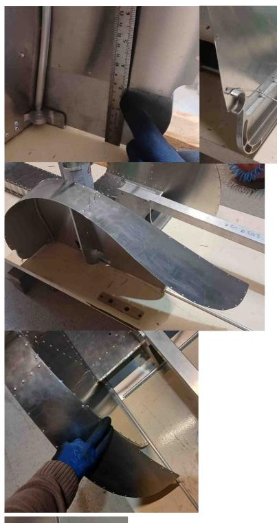
Before fixing the rear of the wheel arch, check that the sheet metal is horizontal.
