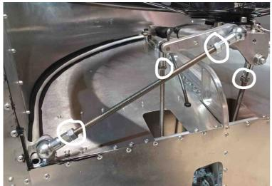
When the train is correctly adjusted, lock all the nuts against the ball joints
