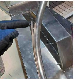
This end (T14 + A8) risks hindering the installation of the bodywork. It is necessary to cut it. The goal is to reduce excess as much as possible. Trace and cut.
