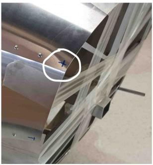
Fix around 8 rivets on the N1 rib
