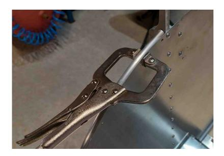
Vise pliers can be handy for holding the tube while drilling and riveting.
