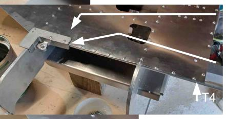
Position **F4** supports, fix it with 2 rivets
