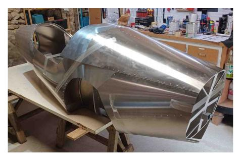
Before tracing the future holes, add adhesive tape to press the sheets together and obtain a final shape.
