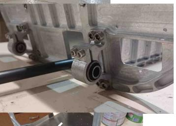
Fix the F10 supports securely with thread lock, grease then place the F9 silent blocks without tightening them for the moment.
