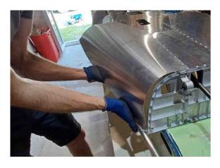
Before continuing riveting, pass the sheet metal under the tube then finish riveting. Repeat the operation on the other side.
