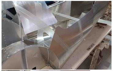
Use tape and don't hesitate to apply tension to press the sheet metal into the correct position.
