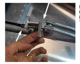
Install the brake cables, remembering for the left one, to add the parking brake pin before inserting it into the housing. The long side of the pin should be facing down The duct stops must be screwed in all the way
