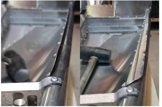
Using a rubber hammer, bend the sheet metal around the tube.
