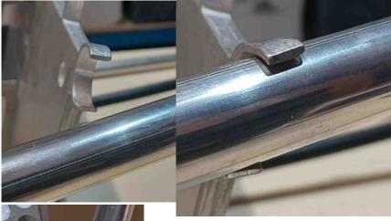
The rear bracket should be bent slightly to accommodate the angle of the tube
