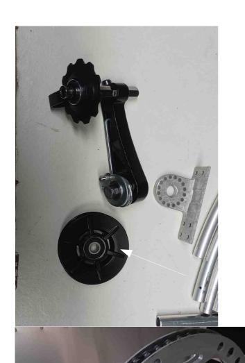
We supplied a front chain tensioner. You can use it or not. It permits to change the crank position without adjusting the chain lenght.
