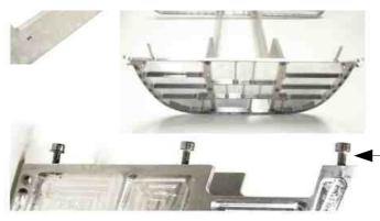
Bolt the rear face N10 with the R 5x10 screws
