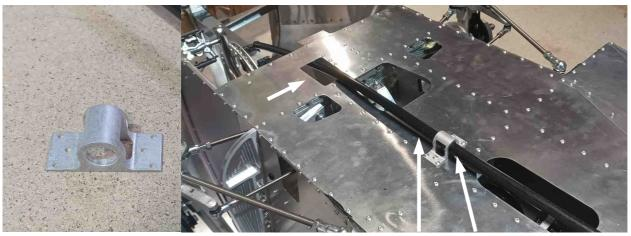
Place the E3 support then insert the Tp3 tube (150cm). It should stop approximately 10cm from the rear wheel axle
