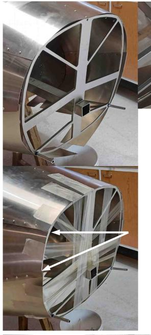
Adjust the position of the forehead rib, then secure it with 4 rivets on the boom
