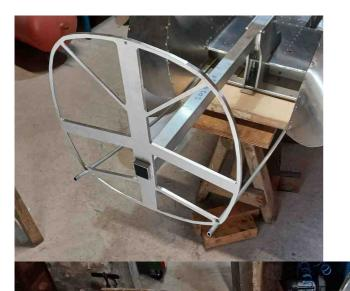
Insert the N1 rib (machined side towards the rear) onto the boom while inserting the two T4 tubes into the holes provided. It is normal to force it, just be careful not to break one of the parts.
