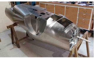
Fix the sheet metal with adhesive tape then add a rivet to maintain the position. By hand, bend the sheet metal around the tube
