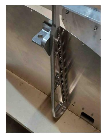
Firmly secure the F3 front suspension supports using thread lock and washers.
