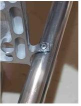
Add rivets to hold the tube in position
