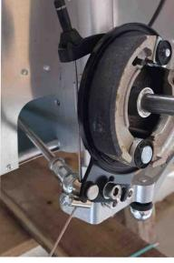
Install the outtercable and its duct stop 1 on the brake lever. Place duct stop 2 in its housing.
