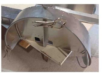
Try to not drill or rivet the tube before it is completely adjusted, it can break the tube. A tolerance of 3-4 mm can be made up when riveting by applying light force.
