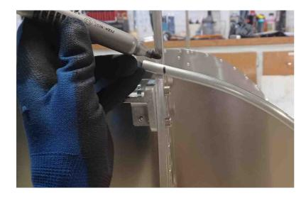
When the adjustment is complete, the excess tube must be cut off. Sand the cutout to remove burrs
