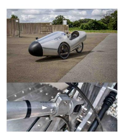
Take the first test drives with caution. Check the effectiveness of the brakes. Balance the braking (right and left) by adjusting the housing stops on the tiller.
