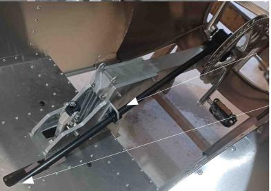
Position the Tp1 tube (60cm) with the rubbers on either side of the E7 guide.
