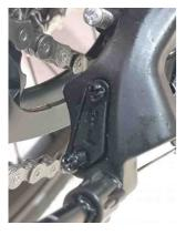
With a small flat screwdriver you can adjust the H and L stops of the derailleur. They define the limits to prevent the chain from going beyond the cassette sprockets.
