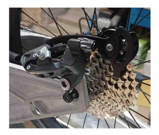
Screw the rear derailleur onto its support The derailler have a stop bolt. Make sure that it takes place without any resistance.
