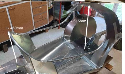
The front must be at 610-620mm from floor to top of the tube
