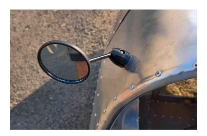
The bottom part of the mirror is fix on the P6x20 head.
