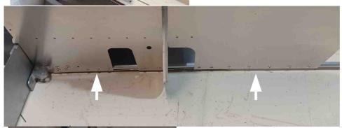
First, fix the bottom with some rivets
