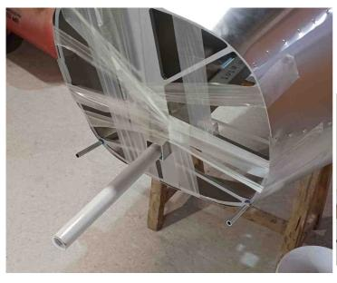
Insert a rod into the boom, you can now easily turn the velomobile onto the trestles
