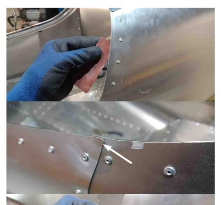
Sand all the burrs and make roundings where there is an angle in the sheet metal.
