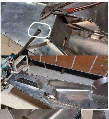
Place the T12 tubes on the two notches, they must be pinched slightly so that they can be inserted
