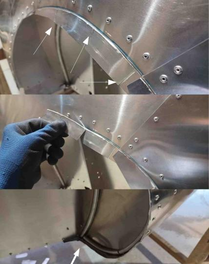
One or two cutting passes are enough, you can then cut small segments and remove them easily by hand.
